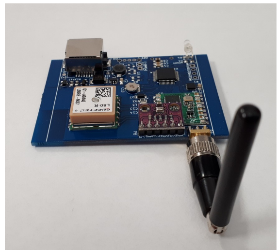
Illustration 2: Orientation of GPS (white-brown box on the left) and radio (right) antennas
