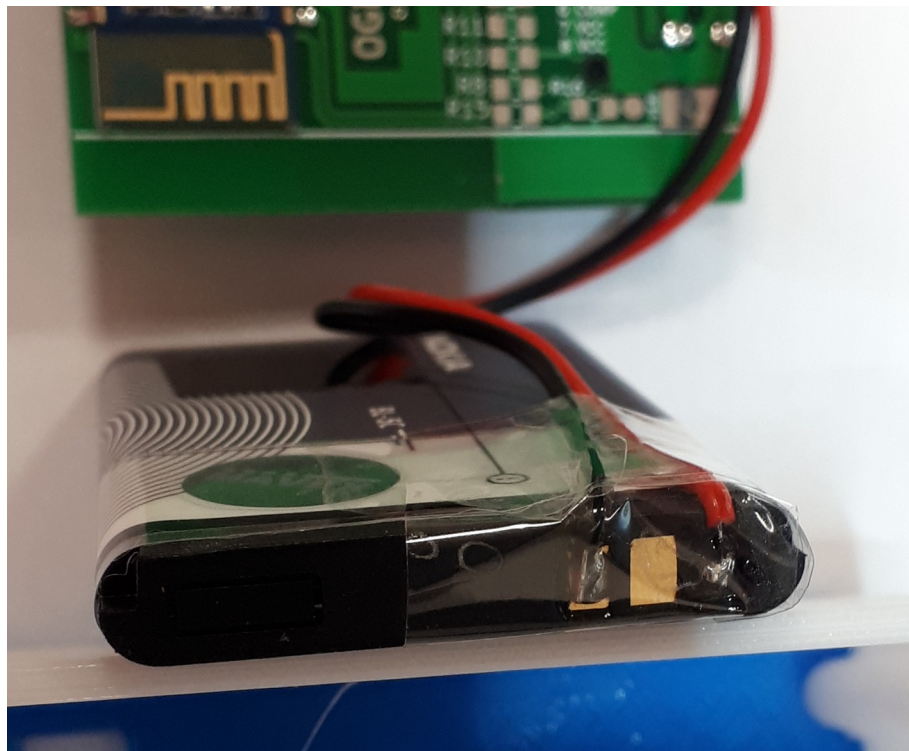
Illustration 9: Wire leads soldered to the battery pads
