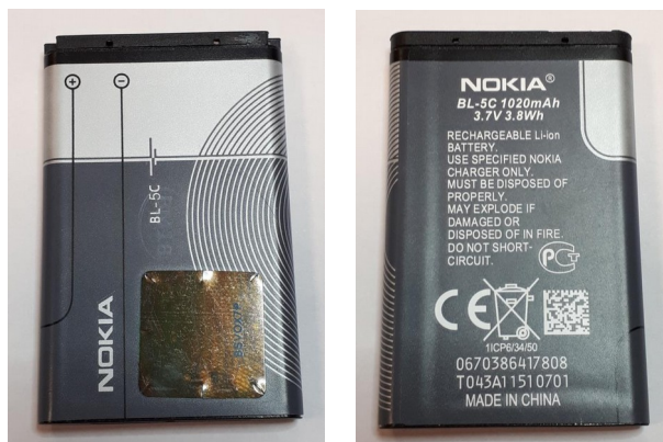
Illustration 6: Internal 1020mAh “Nokia” battery
