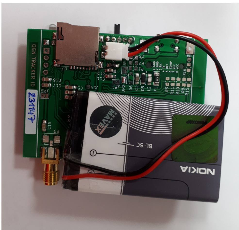
Illustration 7: Battery connected to PCB using a 2.0mm JST connector
