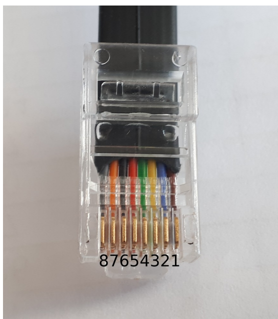
Illustration 4: RJ45 pin denotation with the clip at the bottom side of the plug
