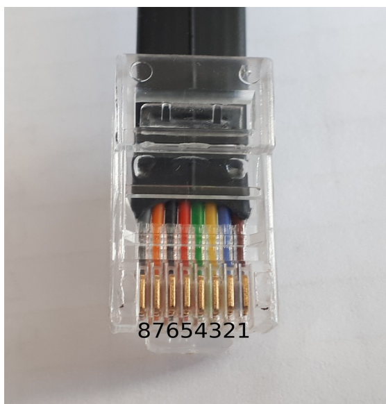
Illustration 4: RJ45 pin denotation with the clip at the bottom side of the plug
