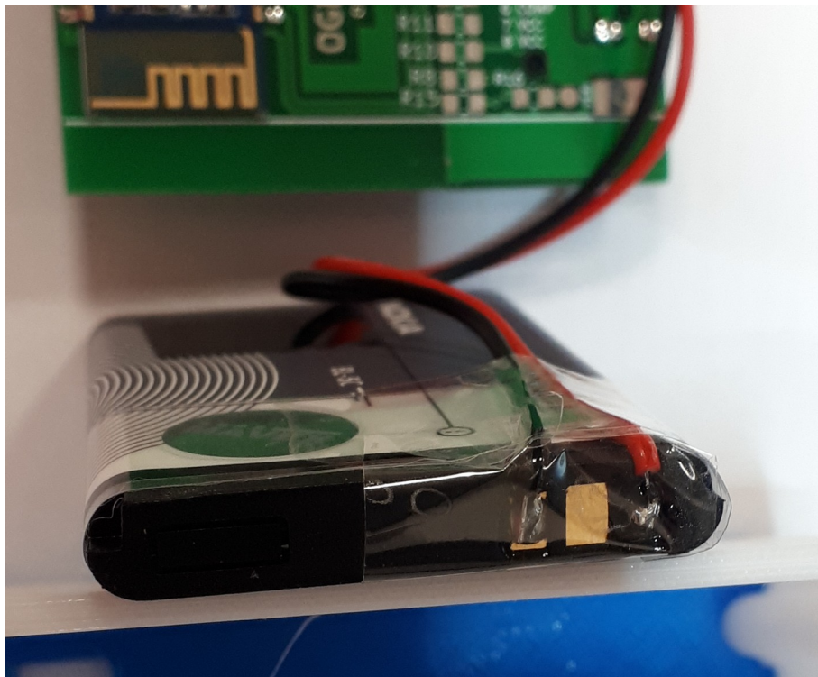
Illustration 9: Wire leads soldered to the battery pads
