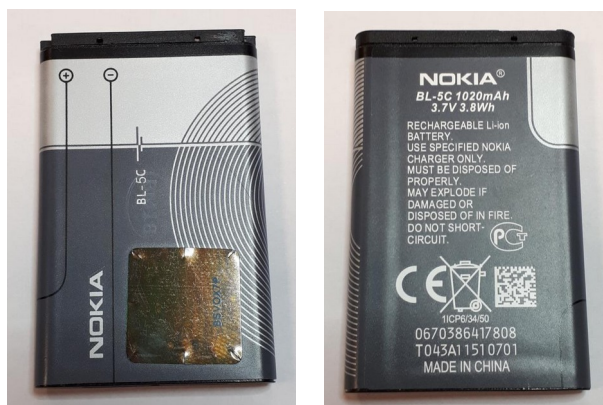
Illustration 6: Internal 1020mAh “Nokia” battery
