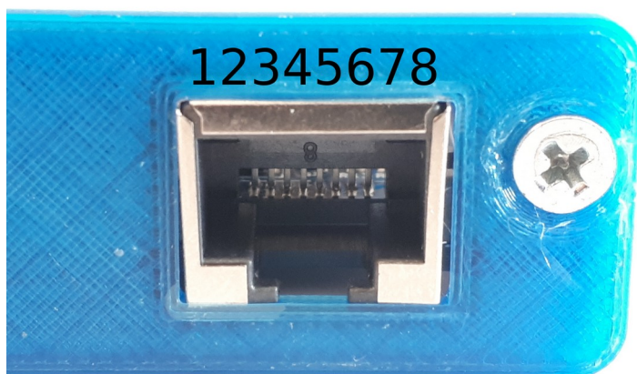
Illustration 5: RJ45 pin denotation on the front face of the unit with the clip at the bottom side
